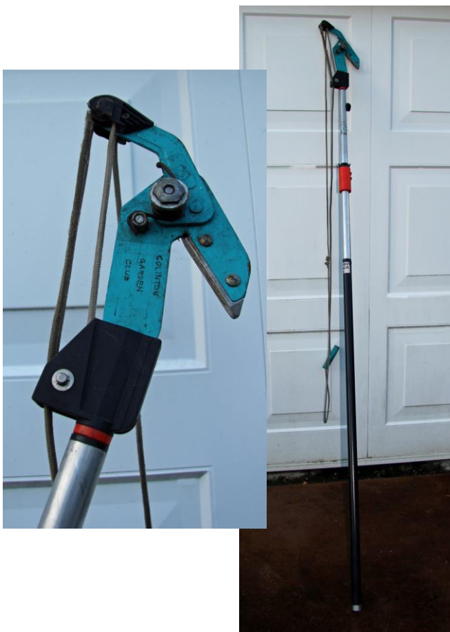
11. Tree Pruning Lopper with (stiff) telescopic handle. Flat blade.
