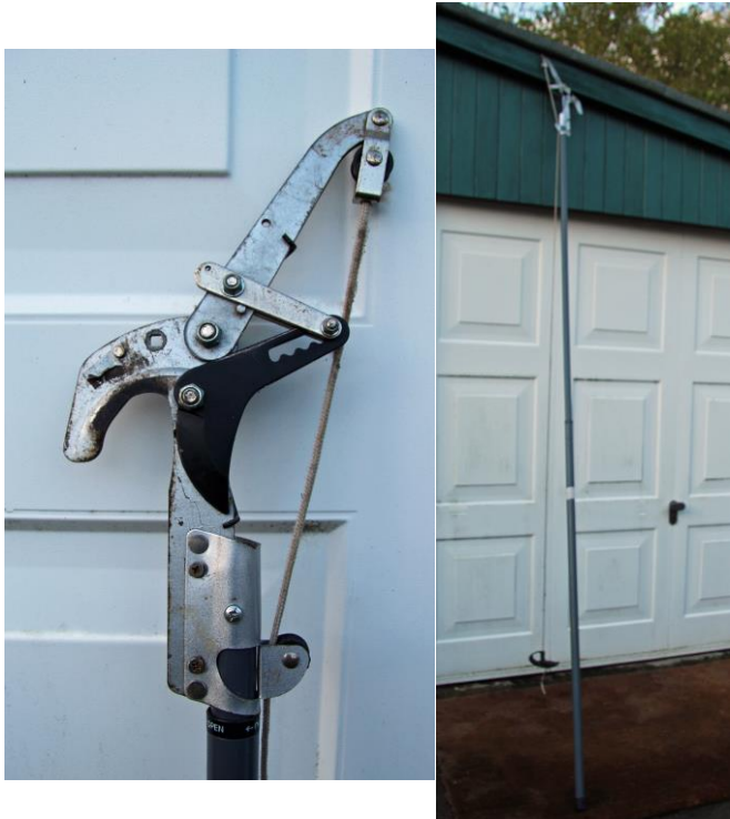
10. Tree Pruning Lopper with long telescopic handle. Hooked blade, ratchet mechanism.
