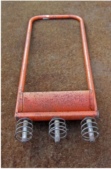
5. Lawn Aerator – 3 hollow tines with springs
